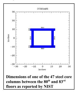
As the core columns progressed to the upper floors, they became smaller in size as seen in the diagram of the columns for WTC floors 80 to 83.<sup>158</sup>
